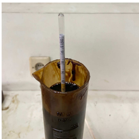
Figure 4. Specific Gravity Testing with a Hydrometer.
