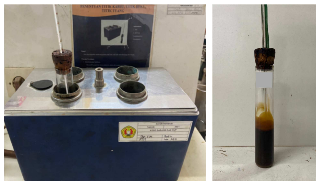
Figure 6. Pour Point Measurement with Water Bath and Thermometer.
