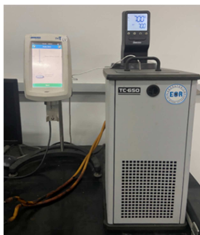
Figure 5. Viscosity Measurement with Brookfield Viscosity Meter.
